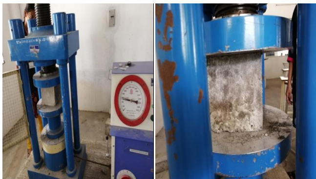
Figure.2 Testing of compressive strength
