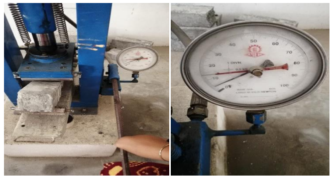
Figure.4 Testing of Flexural strength for concrete
