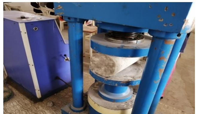
Figure.6 Testing of Split Tensile strength
